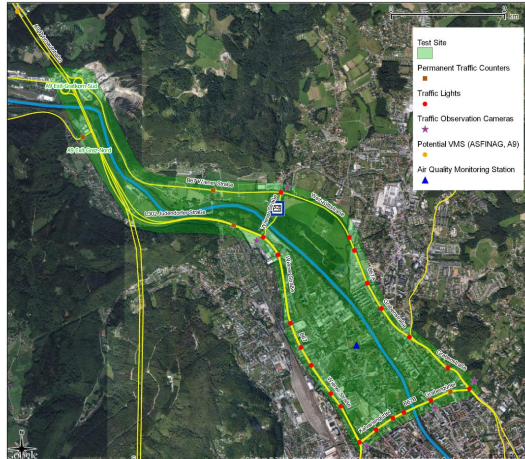
The test site of Graz including existing traffic lights and sensor locations
