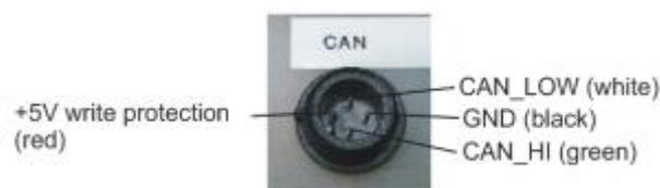
Figure 13: CAN-bus connector
