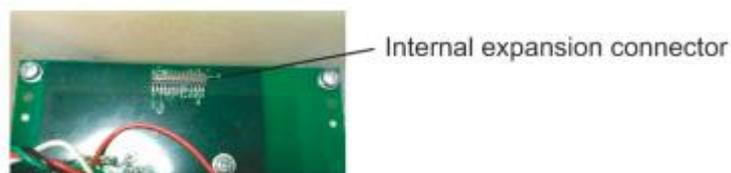
Figure 18: Internal expansion connector
