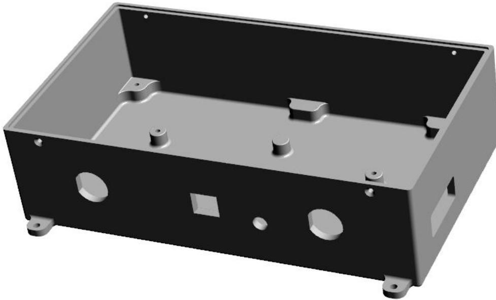
*Figure 9: Lower part of the Traffic unit housing*
