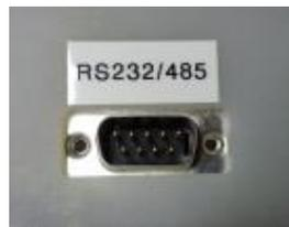
Figure 17: External expansion connector
