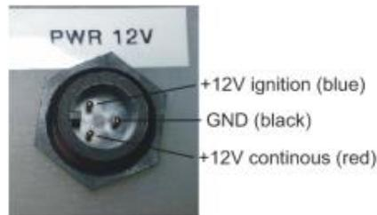
Figure 16: Power supply connector
