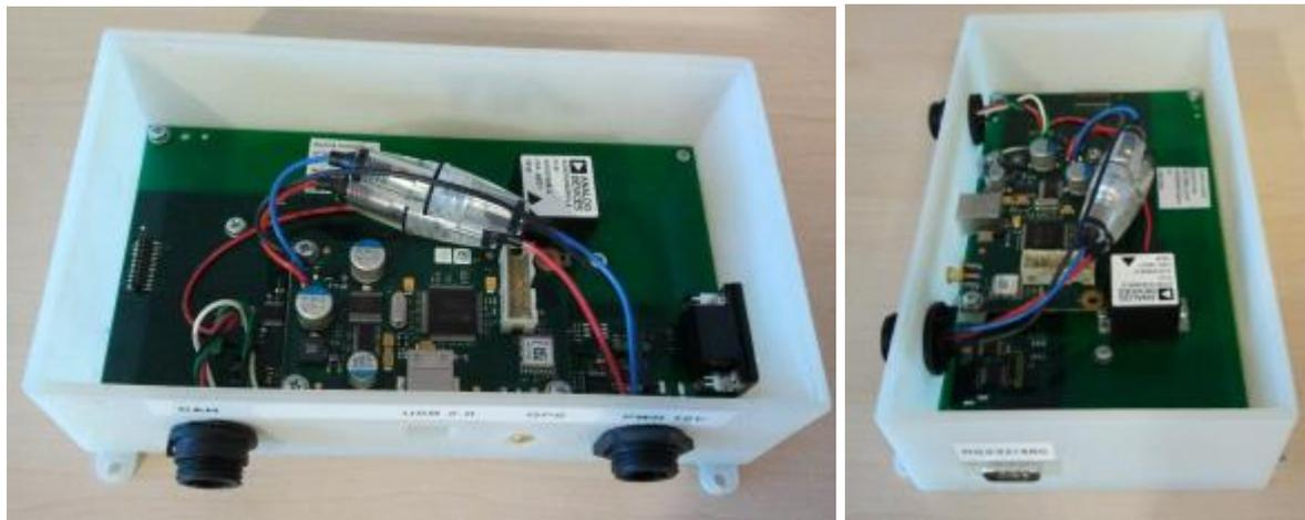
Figure 12: Traffic monitoring unit without cover
