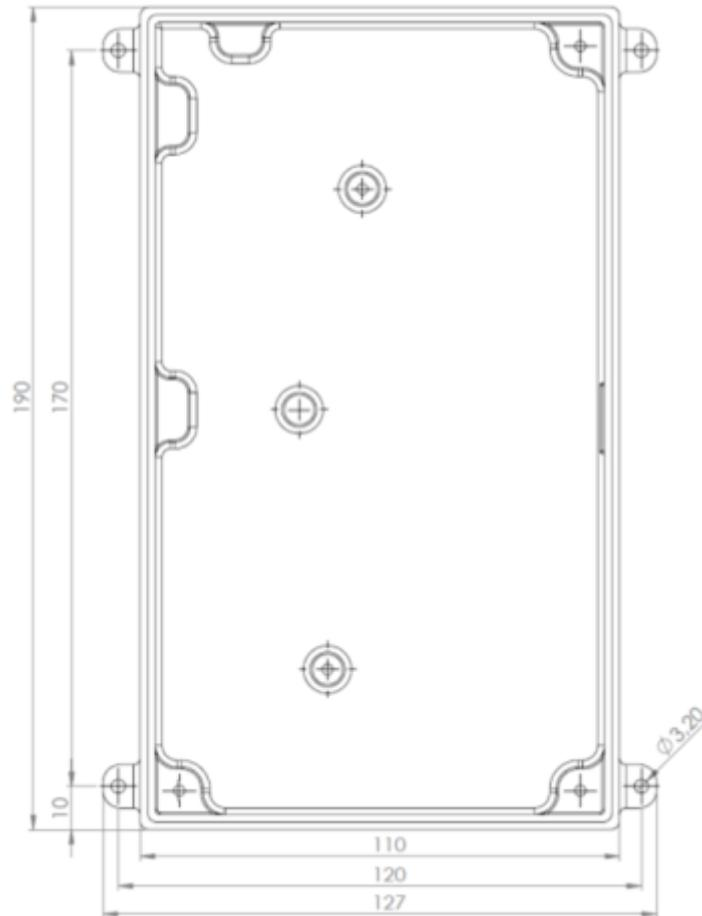
*Figure 8: Dimension of the housing*
