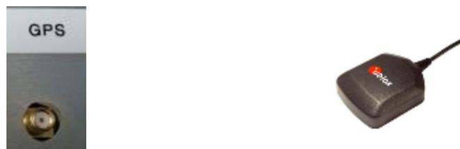
Figure 15: GPS antenna connector and external active GPS antenna
