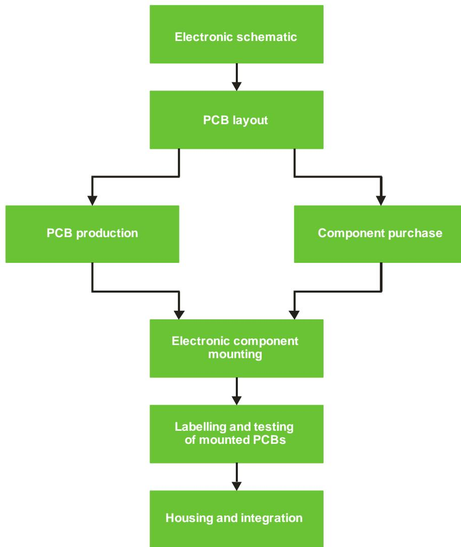
Figure 4: Implementation flow diagram
