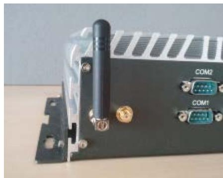
Figure 13: External GSM/UMTS antenna
