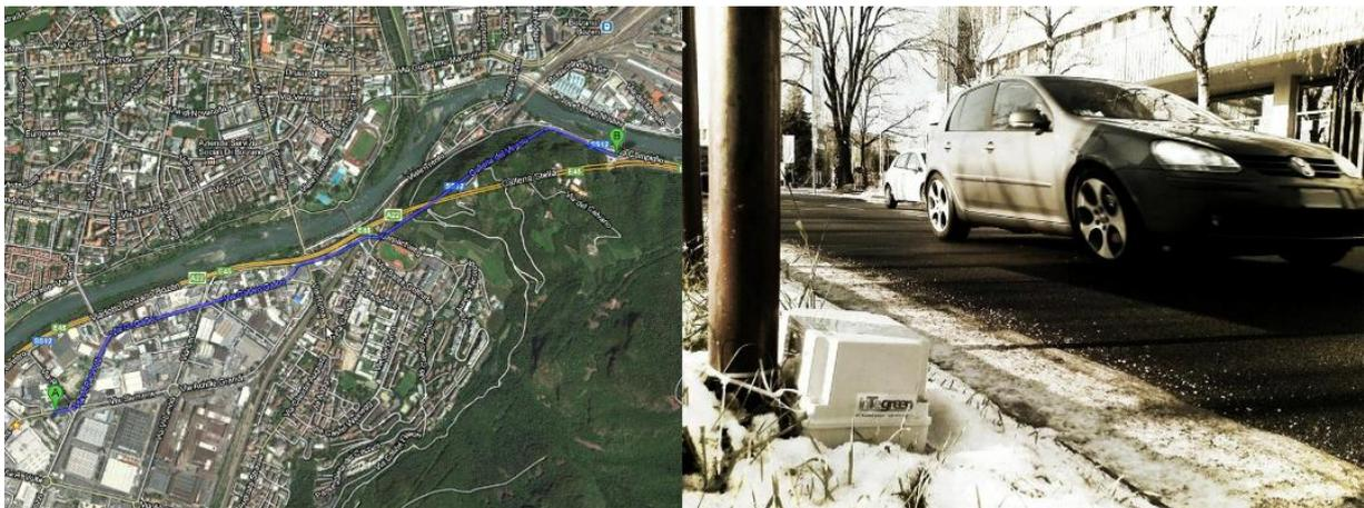
**Figure 5: The travel times measurement campaign: test route and roadside unit.**
